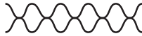
Corrugated sheets riveted together to enable passage of heat transfer fluid between them.
