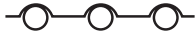
Tubes bonded to formed absorber plate to give increased contact area for good thermal conduction.
