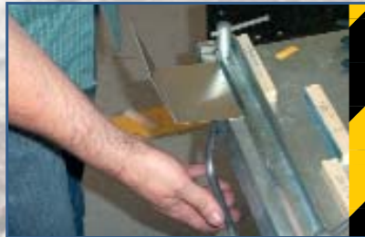
B Bending the aluminium sheet
