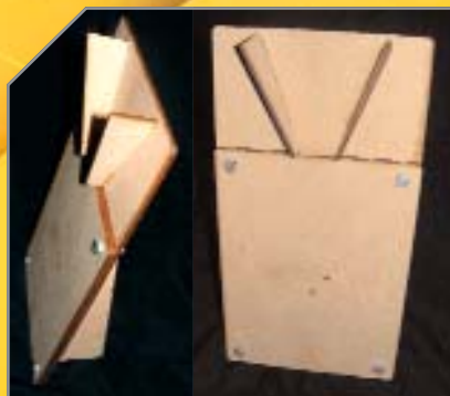
An unusual and clever approach to integrating laser cutting and pewter casting is this innovative laminated mould including runner and mould support legs
