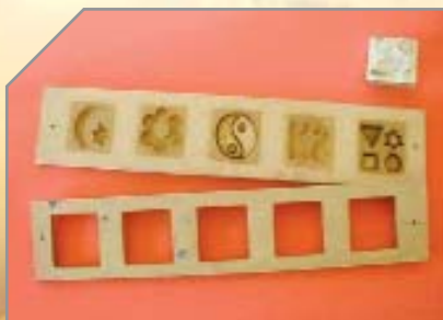
Speedy production of a number of parts is shown here in a strip of milled MDF cavities
