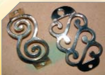
Here the two prototype hair slides have been cast in an open backed MDF mould (milled with a 3mm cutter) and then lightly polished. With care features like the pin holes at the end can be designed into the mould so that they are pre-cast. These castings have also been rolled gently in TEP metalworking rollers to make them curved
