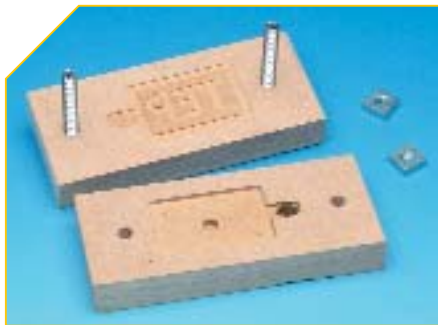
Use of pinch bolts to 'line up' mould layers
