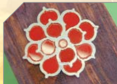
Note the use of cold casting resin to fill cavities in the pewter casting to create an attractive appearance
