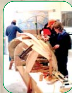
⇒ Traditional boat builders planking the hull
