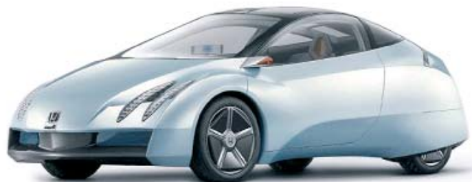
← Concept Honda IMAS This hybrid sports car has two wheels powered by conventional fuel and two wheels powered by electricity.
