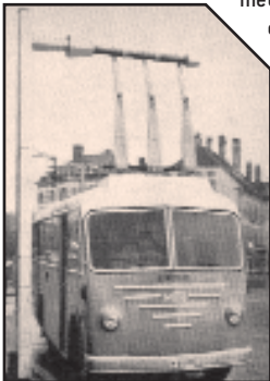
↑ 1950 Gyrobus Electricity to drive the Gyrobus was generated en-route with a fly-wheel of 1500 kg.
