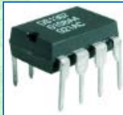
8 Pin PIC 12F629 for use with the Chip Machine. Provides four outputs and two inputs.
