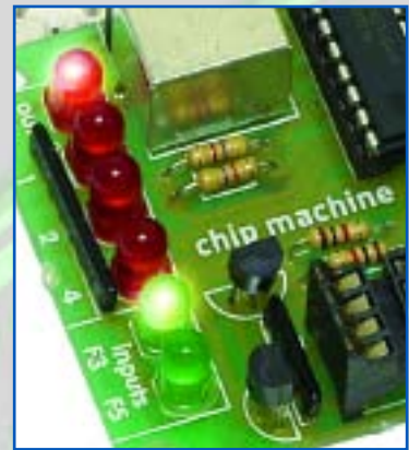
A row of red and Green LED flags on the programmer board indicate the data or instruction entered for each line.
