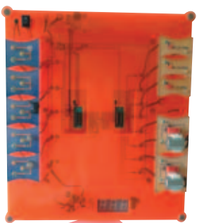
Project with centre removed to show position of PIC chips
