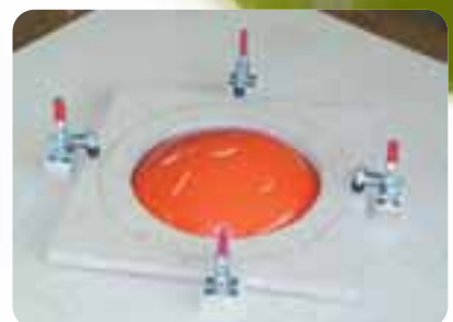
▲ Top of the MDF unit showing the clamps and the dome beginning to form
