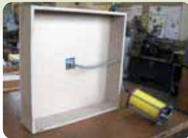
▲ Underside of the constructed MDF unit showing the TEP air reservoir
