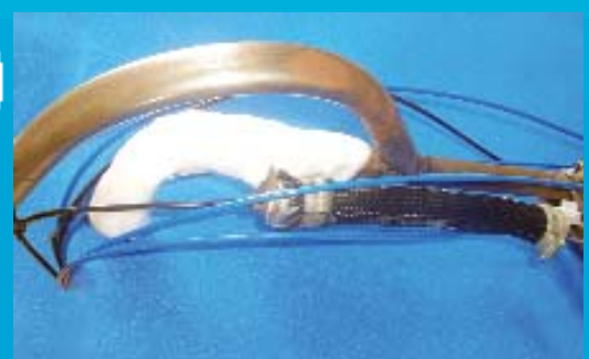
▲ Polymorph has also been used here to replicate a ball joint
