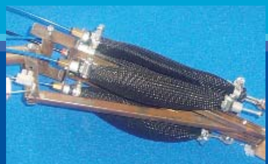
▲ Close up of the Air Muscle - as it inflates the air muscle gets fatter and becomes shorter in length pulling the two end components together
